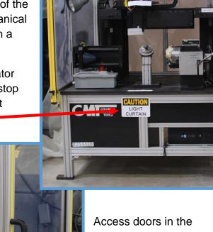
Access doors in the guarding have safety locks. If the doors are opened during the marking cycle, the system will stop.
