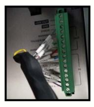
1. Connect the communication cable from the junction box to the back of the laser controller. Each cable will be labeled with a number that will match the numbers on your purchased laser wiring diagram
